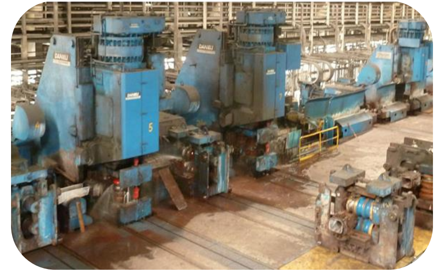
Industrial rolling mills : succession of stands alternating the forming direction
