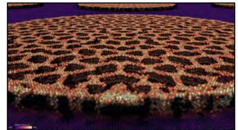
Atomistic stress field of a high angle nano-twist defect by molecular dynamic simulation in a nanolayered intermetallic alloy.
