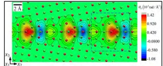
Disclination density field of a tilt grain boundary in Cu [1].
