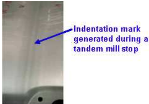
Figure 3: Picture of indentation mark on strip when tandem mill stops at the core of the rolled coil.
